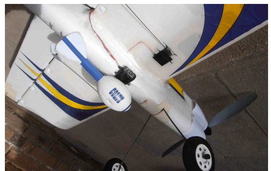
Editor's Typhoon A 31 gram "bomb" held by a simple wire shackle
