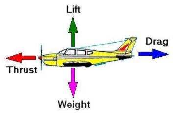
There are many variations on this diagram in various stages of flight. For example, if the engine is not developing power, a component of the Lift vector will replace the Thrust to overcome Drag, but Gravity (weight) always wins! Without Thrust, the plane will descend.
