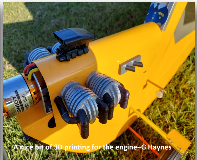
4s Lipos driving a 14x7 prop on a Turnigy motor
