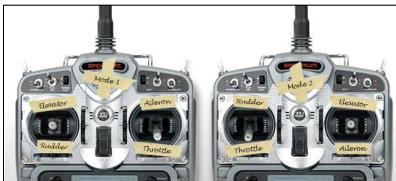
**Mode 1.** Has Aileron and Throttle on the right stick and Elevator and Rudder on the left stick. Having the two primary controls on separate sticks makes it easier to understand the basic functions in the early stages.
