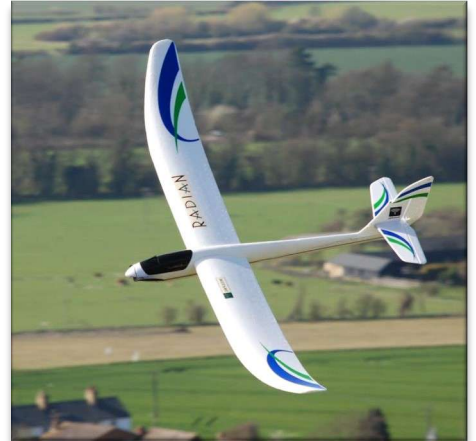
RADIAN. Motor glider, slow flying, great thermal glider. 2m span. 900g RTF.
