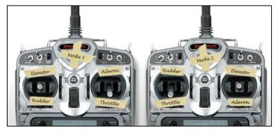
**Mode 1.** Has Aileron and Throttle on the right stick and Elevator and Rudder on the left stick. Having the two primary controls on separate sticks makes it easier to understand the basic functions in the early stages.
