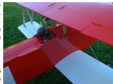
These hard points were secured by small bolts and nuts passing through the wing; then the struts were secured to the angle brackets. Originally I was going to make the struts from hardwood, but ended up using thin aluminium strips. Anyway, the explanation sounds complicated but it was a straightforward although a finicky and time consuming exercise.
