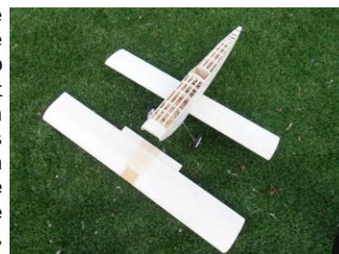
The most complex part of the build was working out and then fitting the cabane and inter-plane struts onto the wings. Perhaps I should have made the wings in the traditional way, that is, spars and ribs, which would have made it easier to incorporate attachment points for the struts. As I chose sheeted foam wings, there were no ribs available. My solution was:
