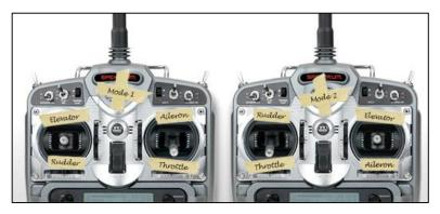
This choice must be made before you make your first flight. HMAC teaches primarily Mode 1. (Aileron and Throttle on the right stick, Elevator and Rudder on the left). Having the two primary controls on separate sticks makes it easier to understand the basic functions in the early stages. Once you start on a particular Mode it is very hard to change over to the other Mode. Mode 1 is the way that most people
